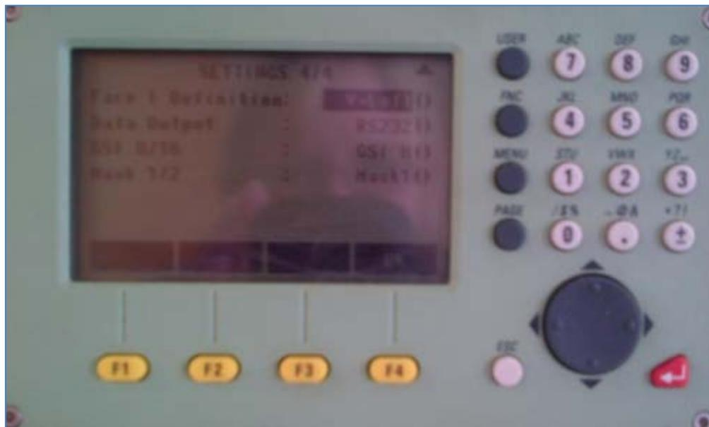
3. Within the main menu use the page button to access page 2 of 3 select **Option 6 'COMM'**, use the arrow keys to highlight and then press the Red enter button to accept, or select **F2**.
